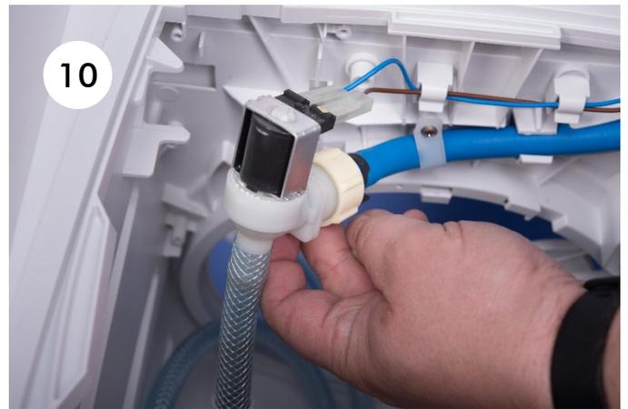
10. Disconnect the connector from the solenoid valve.
