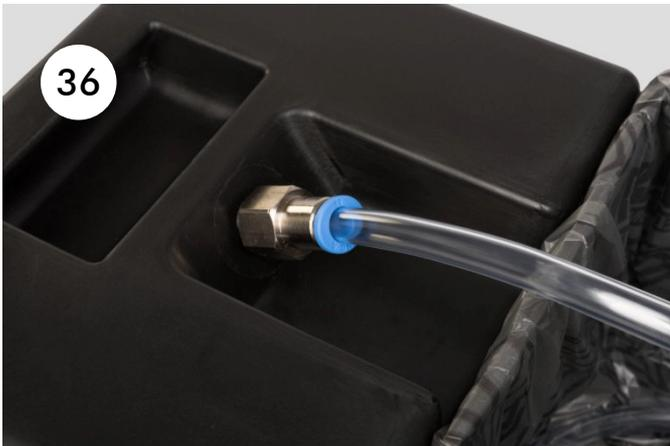
36. Insert the hose into the hose connection of the cassette. Check that it is in tight contact with the silicone sleeve and that there are no kinks, beads and that it has a downward slope. If this is not the case, you should shorten the hose again by a few mm.
