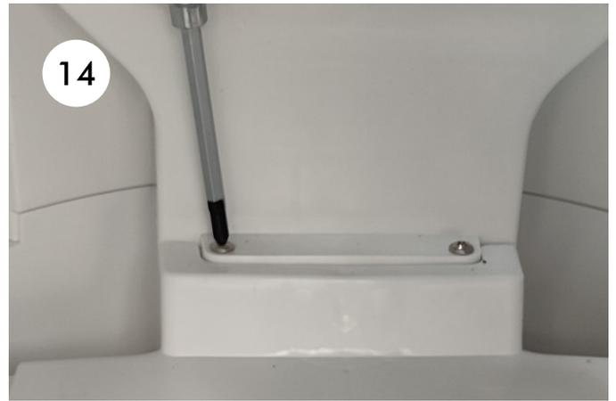
14. Loosen the two screws that secure the cover in front of the back wall of the service compartment.
