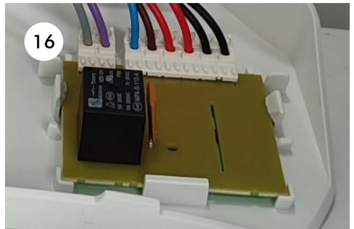
16. Remove the printed circuit board from its holder by pushing the three fastening clips outwards.
