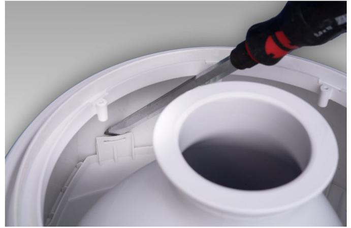
21. Loosen the bowl by carefully pushing one of the two rear fastening clips forward with a screwdriver with a long shaft. If the bowl still does not pull off well, loosen the second rear fastening clip in the same way.
